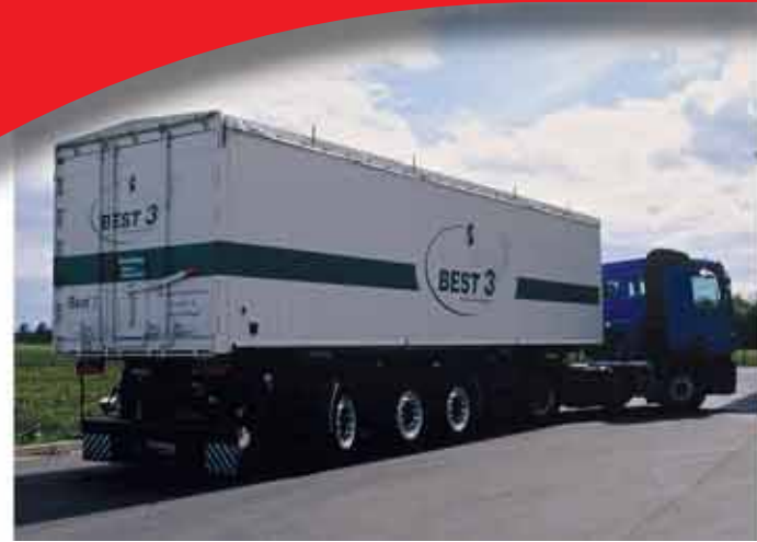
Vehicle type: End-dump combo-trailer (OPTIMATIC) Perm. total weight: 39,000 kg Empty weight: Approx. 7,130 kg
