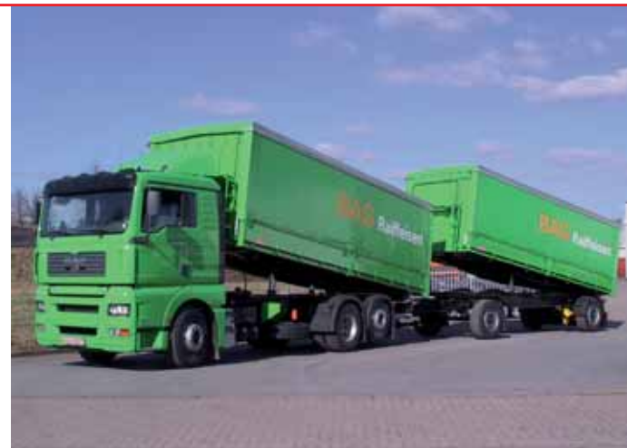
Vehicle type: Three-way pallet dump vehicle Perm. total weight: 26,000 kg motor coach and 18,000 kg trailer
