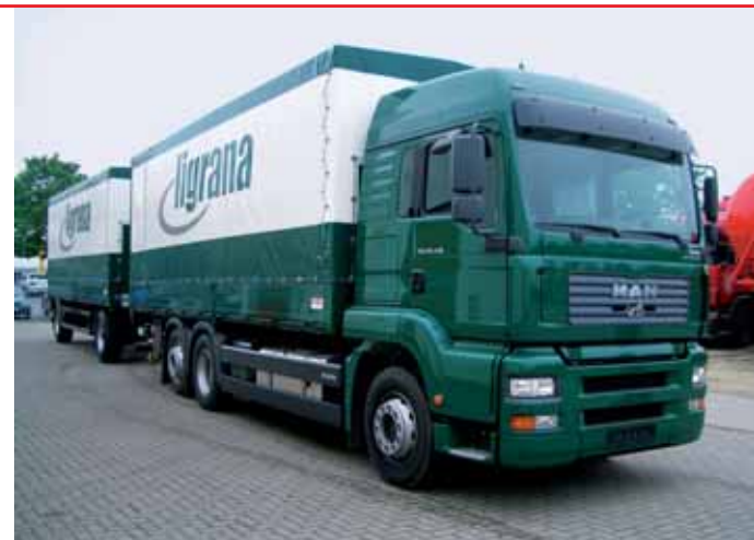
Vehicle type: Big-bag pallet setup Perm. total weight: 26,000 kg Design weight: Approx. 2,830 kg
