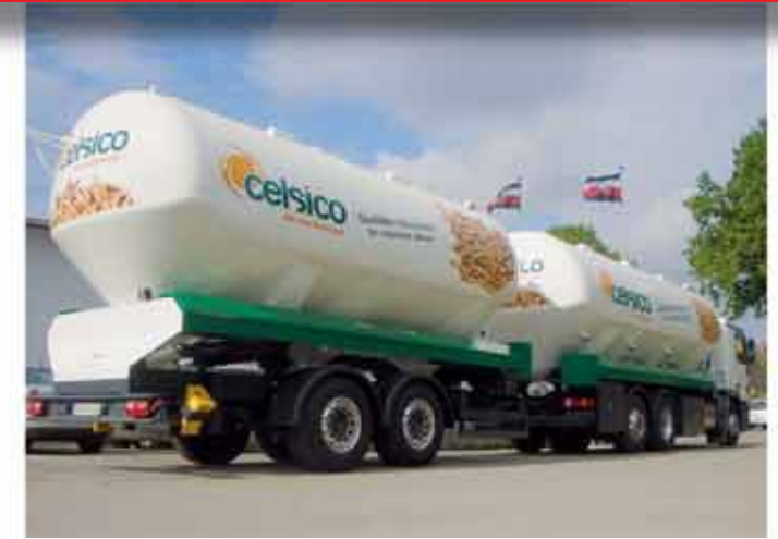
Vehicle type: Hopper train with on-board weighing Perm. total weight: 26,000 kg/18,000 kg
