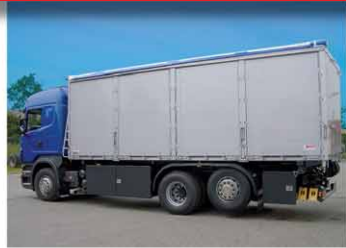
Vehicle type: Two-way combo dump setup Perm. total weight: 26,000 kg Design weight: Approx. 3,430 kg
