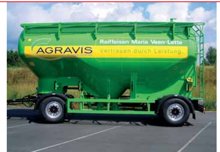
Vehicle type: High-pressure hopper trailer Perm. total weight: 18,000 kg Empty weight: Approx. 3,430 kg
