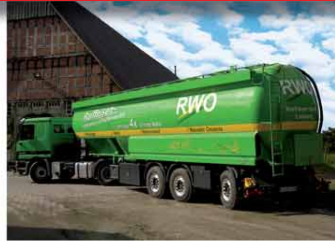
Vehicle type: 3-axle high pressure hopper trailer Perm. total weight: up to 39,000 kg Empty weight: Approx. 7,130 kg
