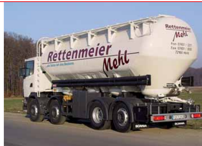
Vehicle type: High-pressure hopper setup Perm. total weight: 32,000 kg Design weight: Approx. 2,790 kg
